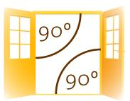
IF DOORS ARE IN DIFFERENT HEIGHTS OR THERE IS A GAP BETWEEN THEM, ADJUST 3 SCREWS ON DOOR HINGES.
